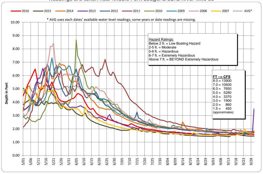
Note: This hydrograph is a very general guide for predicting flows. The lines merely connect daily flow readings. Considerable fluctuation can occur daily, especially on very warm days and after high-intensity rain storms.
