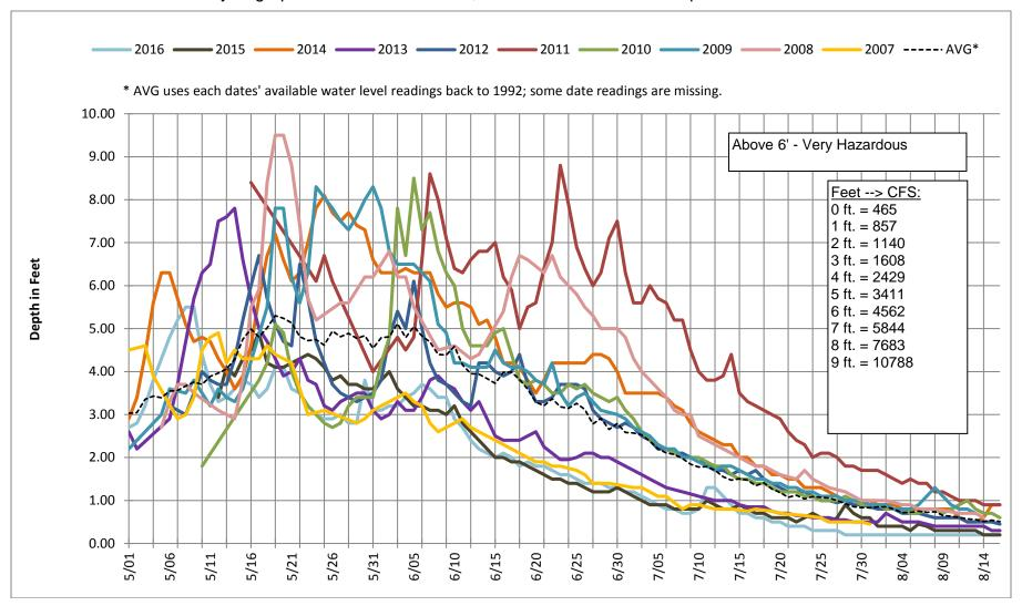
Note: This hydrograph is a very general guide for predicting flows. The lines merely connect points which were read on the dates shown. Considerable fluctuation can occur daily, especially on very warm days and after high-intensity rain storms.
