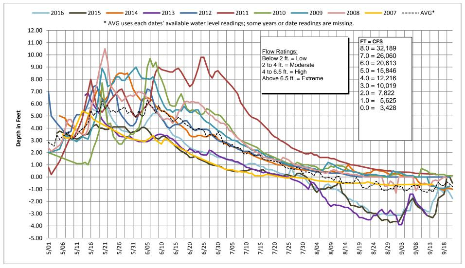
Note: This hydrograph is a very general guide for predicting flows. The lines merely connect depth points which were read on the dates shown. Considerable fluctuation can occur daily, especially on very warm days and after high-intensity rain storms.
